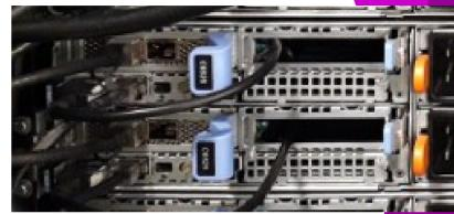
• Removal of 2nd PCIe riser to let USB cable through
