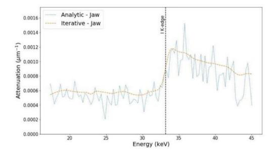
Comparison of reconstructions with FDK and with a **novel iterative algorithm** developed using CIL
