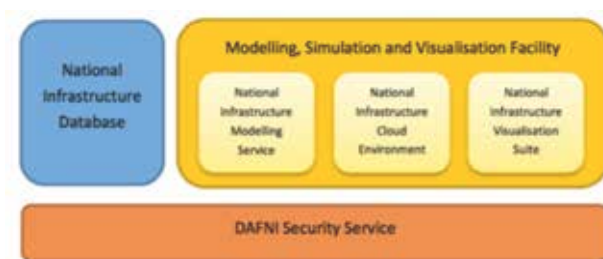
Figure 1: DAFNI Core Capabilities. The five core components are shown here encapsulated by the initial separations that were defined as Modelling Simulation and Visualisation Facility (MSVF) and National Infrastructure Database(NID)
