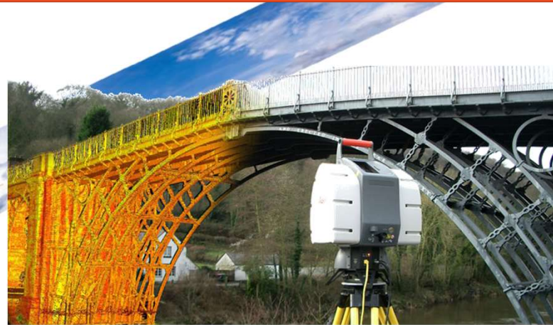
Fig 4. Digital twins of a bridge using 3D scanner
